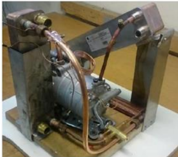
100g of R290 10 kW heating capacity 33cc compressor
